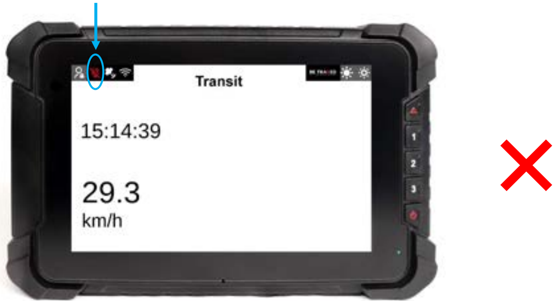
Figure 2 - Red power indicator light: device not powered
